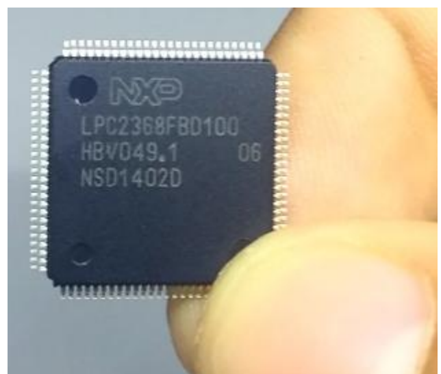
Fig. 10. Encapsulamento do LPC2368FBD100[13].
